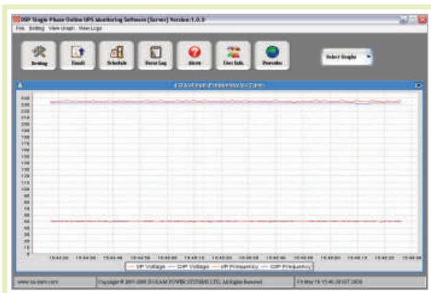
**View Graphs :** User is provided with different Graphs: • Input Voltage, Output Voltage, Input Frequency, Output Frequency plotting vs. Time • Battery Voltage vs. Time • Load (%age) vs. Time. User has dynamic graphs through which users would be able to even drag graphs to zoom at particular interval of Time. I/P, O/P Voltage and I/P, O/P Frequency Vs Time
