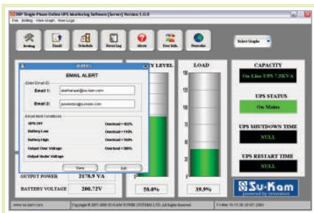
**Email Notification :** User can configure Power Manager to send Email Alert message up to 2 people when an Alert occur on various conditions like UPS OFF, Battery Low, Battery High, Output Over Voltage, Overload etc.
