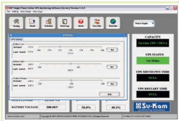
**UPS Settings :** Power Manager provides the way to set UPS Settings (like Battery Low, Battery High and Output Voltage). It provides flexibility in the sense that user can have control on UPS.
