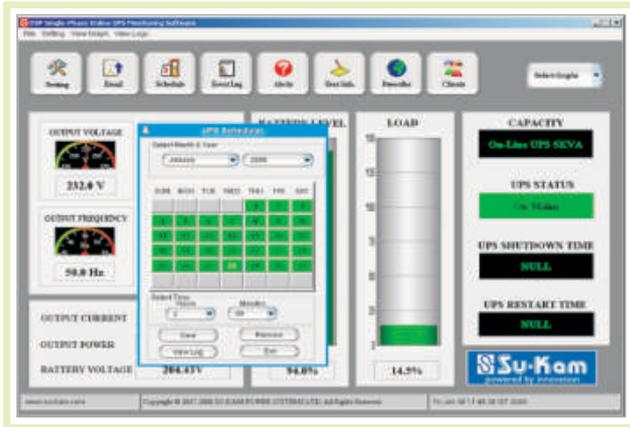
**UPS Schedule :** With Scheduler, user is able to schedule, shut down of all segments of UPS load at a specified time. It provides the flexibility to user, to have full control on UPS.
