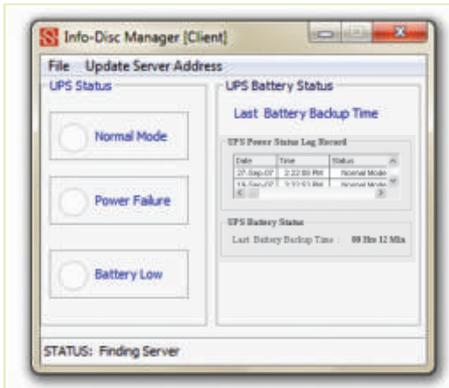
The Su-Kam Digital Line Interactive UPS RS232 monitoring software "Info Disc Manager" is compatible with almost all popular operating systems with best reliability. An easy to install auto run software CD and DB-9 Communication connector cable is to be connected to facilitate convenient interfacing of PC with UPS.
