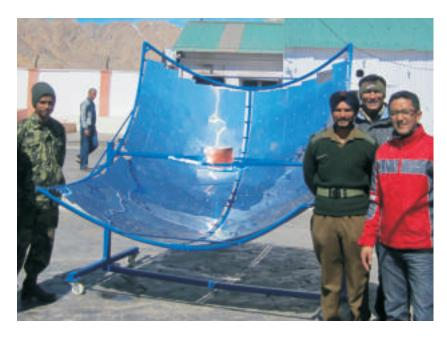
1.4 m<sup>2</sup>, 2.5 m<sup>2</sup> or of 4 m<sup>2</sup> of elliptical or parabolid shape.
